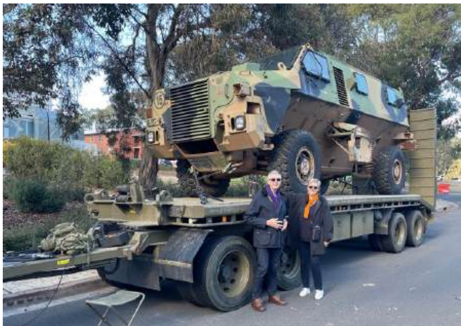
Stuart and Glenda with a Bushmaster, displaying its usually hidden special triangular shaped lower body which helps protect the occupants from IEDs
